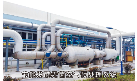
System of Fermentation Sterile Air Pretreatment (SAS)
